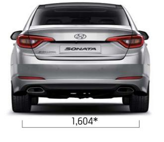
\*Wheel tread • 16" alloy wheel (Front/rear) : 1,614/1,621 • 17" alloy wheel (Front/rear) : 1,602/1,609 • 18" alloy wheel (Front/rear) : 1,597/1,604
