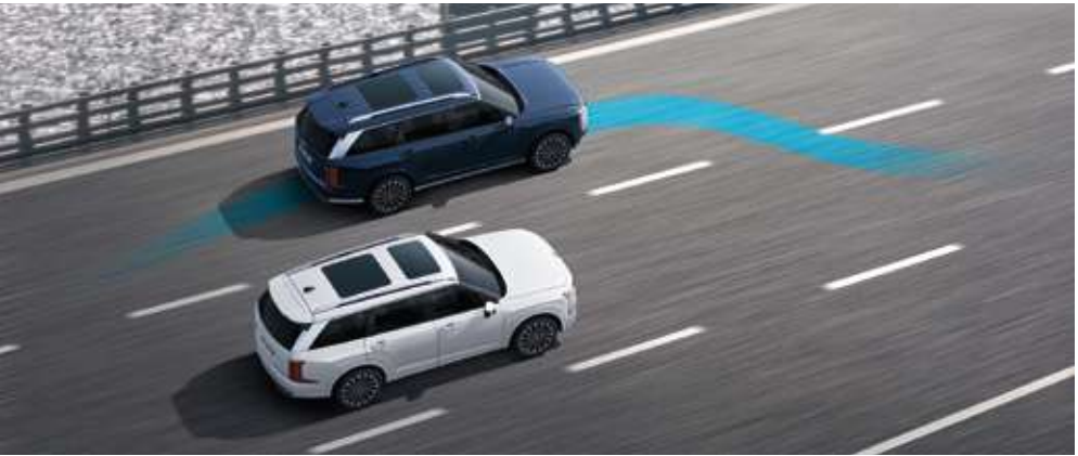
During lane change, this function provides a quick yaw response and improved cornering stability.
