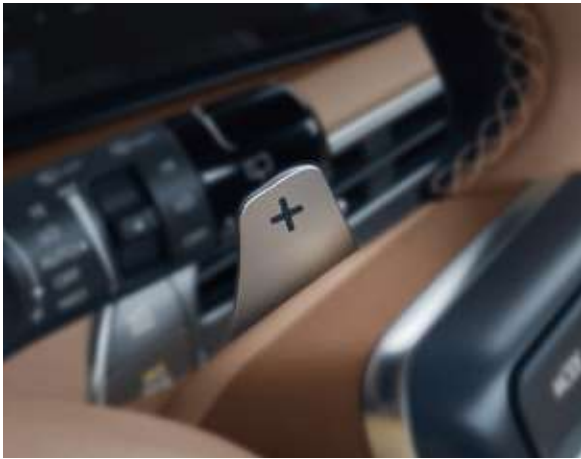
Stay Mode Paddle Shift-Regenerative Braking Mode * Stay Mode will not operate if any of the following conditions occur: if the State of Charge (SoC) is below 35%, the low fuel warning light is on or the main battery relay is off, or if the vehicle is not in Park (P).
