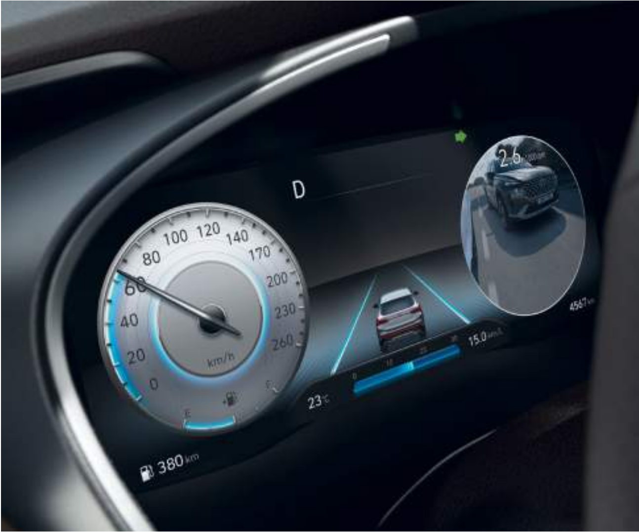
12.3" Full LCD Cluster & Blind-Spot View Monitor (BVM)
