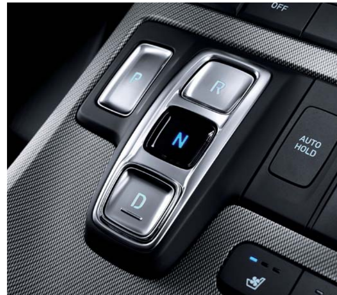
8-speed shift-by-wire automatic transmission
