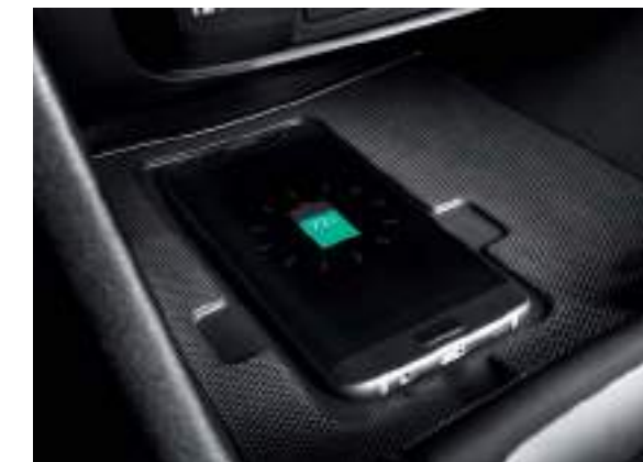
Smartphone wireless charging system
