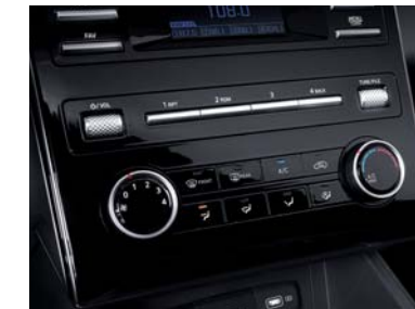
Manual air conditioning system
