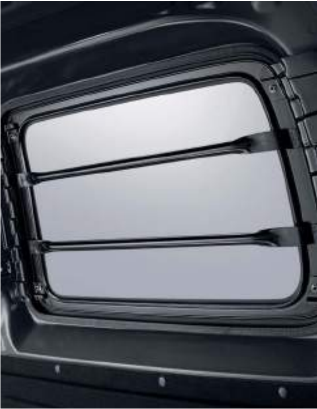
Window security bars
